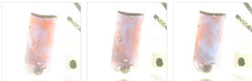
Figure 1.7. 3D waves' formation in the Belousov-Zhabotinsky reaction, which was observed in a test tube of 1 cm in diameter (reaction volume is 2.5 ml) and after 5 minutes' continuous mixing of components by a magnetic stirrer (Fisher Scientific Isotemp Magnetic Stirrer 60-1200 Rpm) with 150 rot/min.
