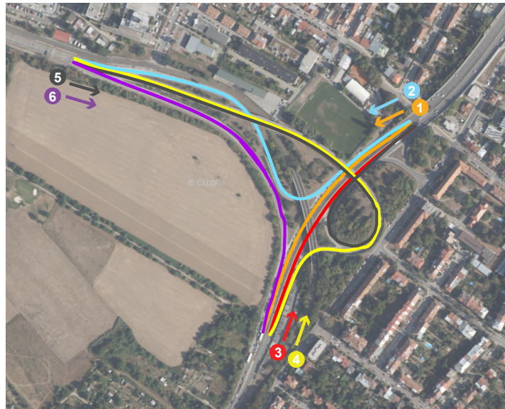
Figure 1.1: Scheme of the interchange number 2432A012 (road I/42 \times II/384, Žabovřeská \times Kníničská street).
