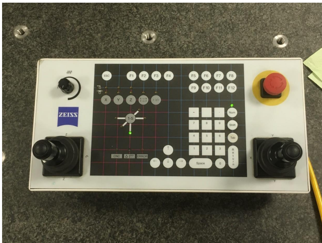
Obr. 3.7 Riadiaci panel CMM Zeiss UPMC 850 Carat
