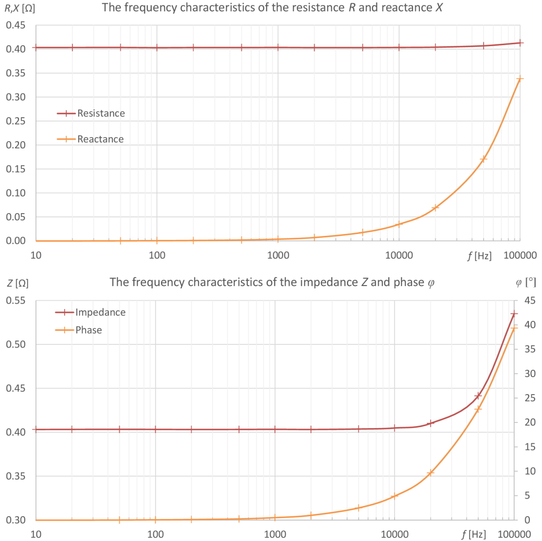
Fig. 3.18: The frequency characteristics of the multiplexer’s resistance, reactance, impedance, and phase.
