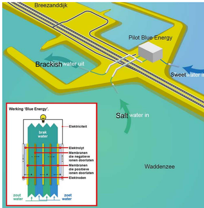
Figure 10: Water flow of the pilot plant on the Breezanddijk in relation to the Wadden Sea (REDstack ©2023).
