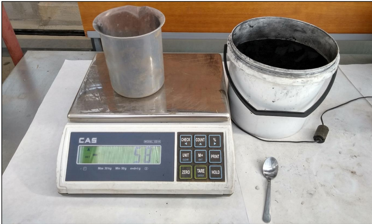
Figure 4.4: Laboratory instruments used to measure and add up the amendments to the soil. In addition, a plastic spoon was also used for nanoiron amendment processing
