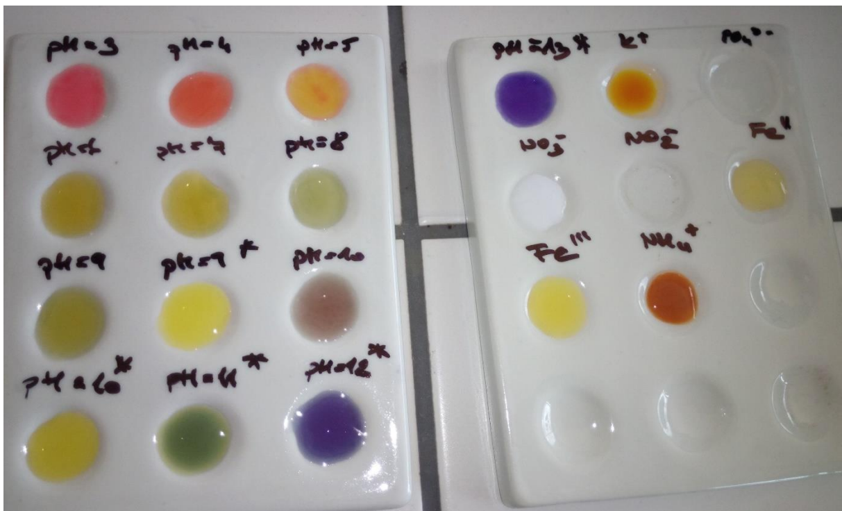
Figure 14B. Drip plate with ion and pH samples after reaction with appropriate reagents (pH with star mark means use of pH reagent with range 9-13)
