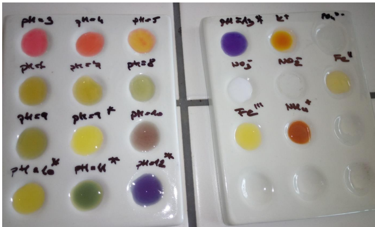
Figure 23B. Drip plate with ion and pH samples after reaction with appropriate reagents (pH with star mark means use of pH reagent with range 9-13)
