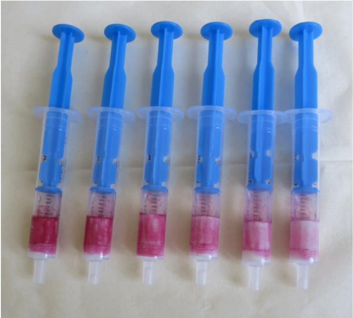
Figure 23. Photography of Ni(II) calibration using true LIS tests with the rectangular detection part
