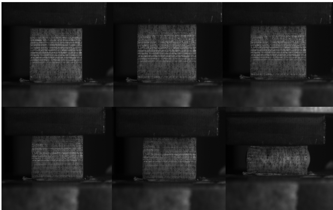
Figure 40. Deformation process in time on images that were used for DIC analysis
