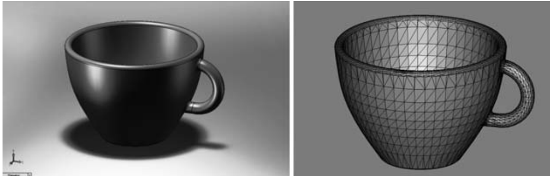
Figure 1. A CAD model on the left converted into STL format on the right
