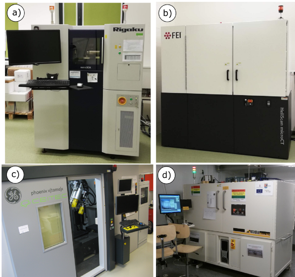
Figure 3.1: CT machines used in the thesis: a) RIGAKU nano3DX, b) Thermo Fisher Scientific HeliScan, c) GE phoenix v|tome|x L240, d) Zeiss Xradia nanoXCT-100.
