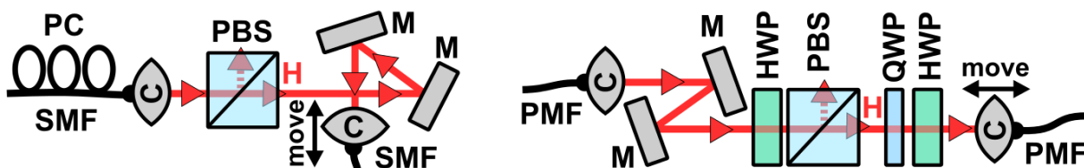
Figure 3.19: Schemes of air gaps (AGs) in different configurations: left – “triangle” shape using single-mode optical fibres, right – “Z” shape using polarization maintaining optical fibres. SMF – single mode optical fibre (type 780-HP), PMF – polarization maintaining optical fibre (type PM780-HP), C – collimating lens, PC — polarization controller, M – mirror, PBS – polarizing beam splitter used as polarizer, move – linearly translating stage for AG length alignment, HWP – half-wave plate, QWP – quarter-wave plate, H – horizontally linearly polarized state of light.
