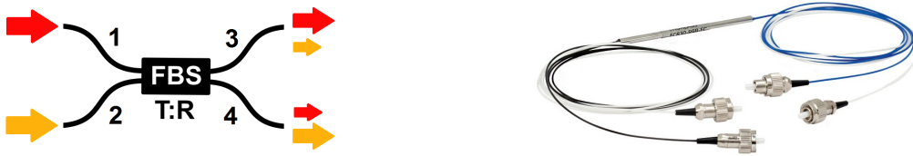
Figure 3.9: left – general scheme of fibre beam splitter (FBS), 1,2 – input ports, 3,4, – output ports. right – photo of the typical FBS [adopted from Thorlabs.com].
