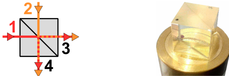
Figure 3.4: left – scheme of a beam splitter (BS) with clarified mode notation, 1,2 – input modes, 3,4, – output modes; right – Photo of a typical cube BS.
