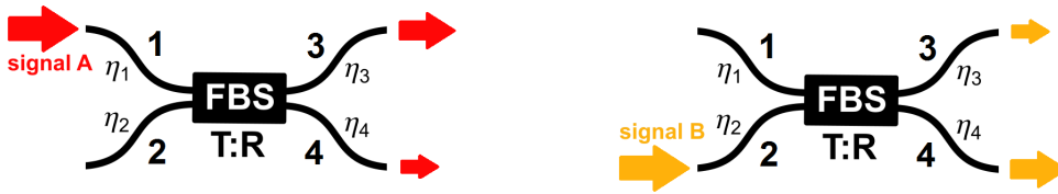
Figure 3.11: Measurement of fibre beam splitter splitting ratio R : T , 1,2 – input ports, 3,4, – output ports, \eta – efficiency / transparency of the port.
