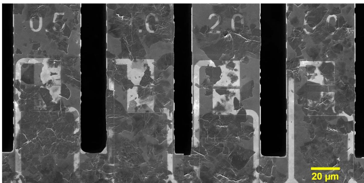
Figure 36: SEM image of graphene oxide flakes on chip.
