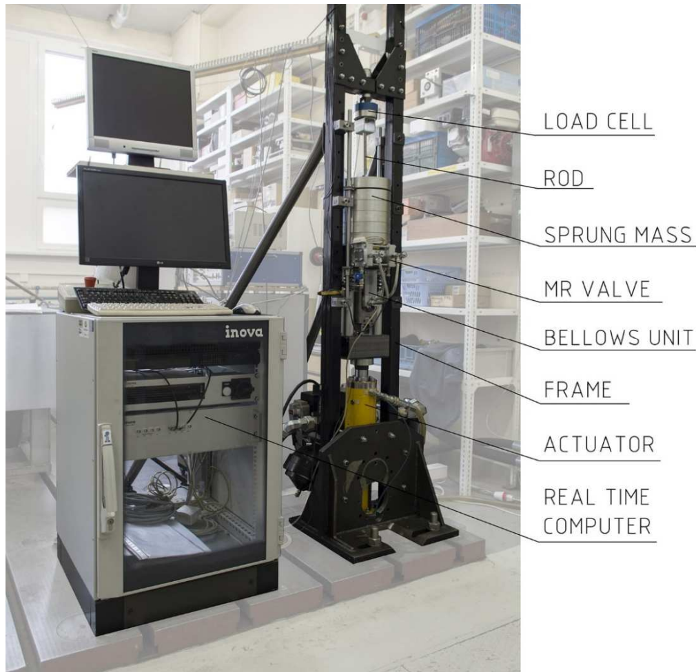
Fig. 68 Demonstrator configuration for the F-v dependency measurement
