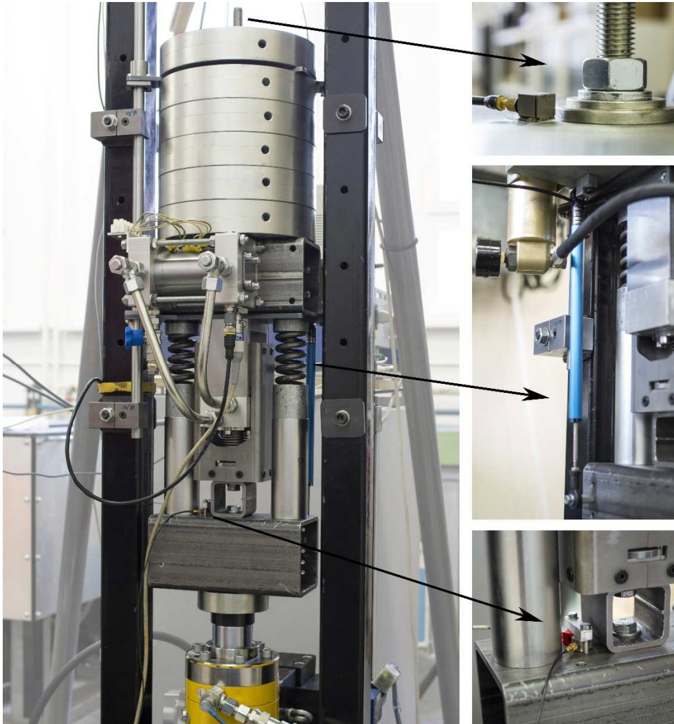
Fig. 67 Demonstrator for the experimental strut vibration isolation properties verification
