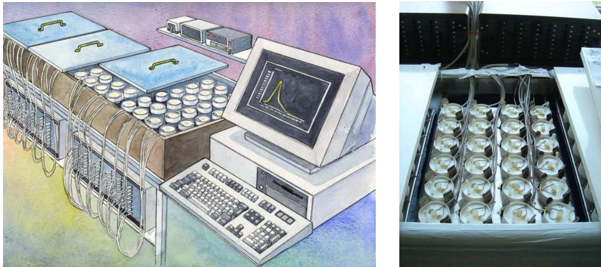
Fig. 14 Schematic and photograph of Respicond device
