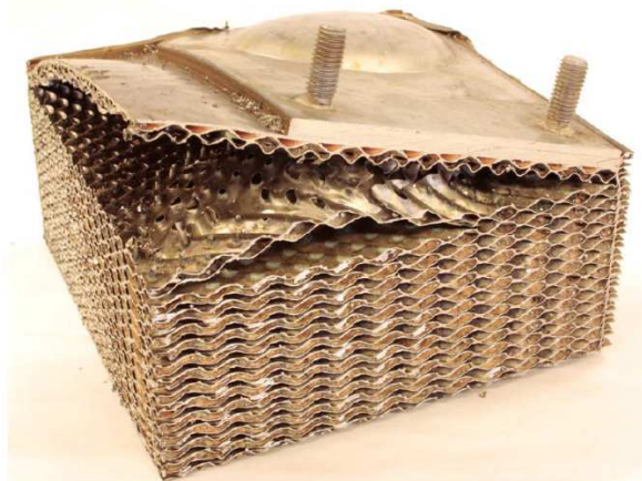
Figure 27 – Cut out section of the unit showing plastic deformation within the unit
