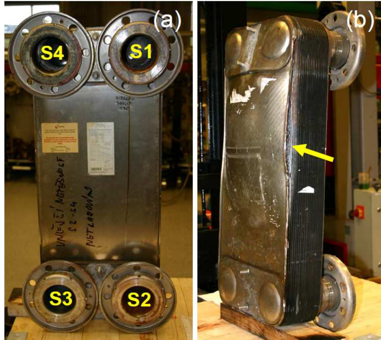
Figure 26 – The researched heat exchanger seen from frame plate (a) and pressure plate (b)
