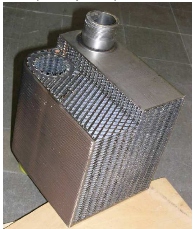
Figure 23 – Sample of exchanger CBH76-80M
