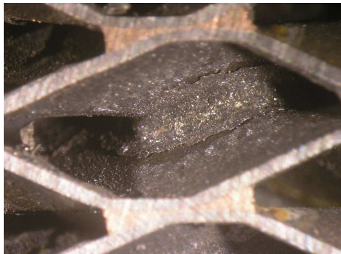
Figure 25 – Joint on secondary side
