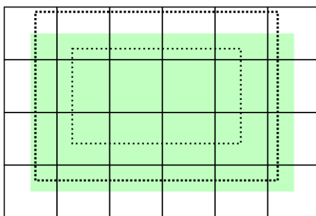
Figure 3.11: Chunks updated by fluid dynamics. The inner dotted rectangle represents the direct view into the world. The outer dotted rectangle represents the area that is required to be active and continuous (the view extended by fixed-size padding on all sides). All standard chunks that the outer rectangle overlaps must be loaded and continuous, the update chunks inside it (green) will be updated by fluid dynamics.
