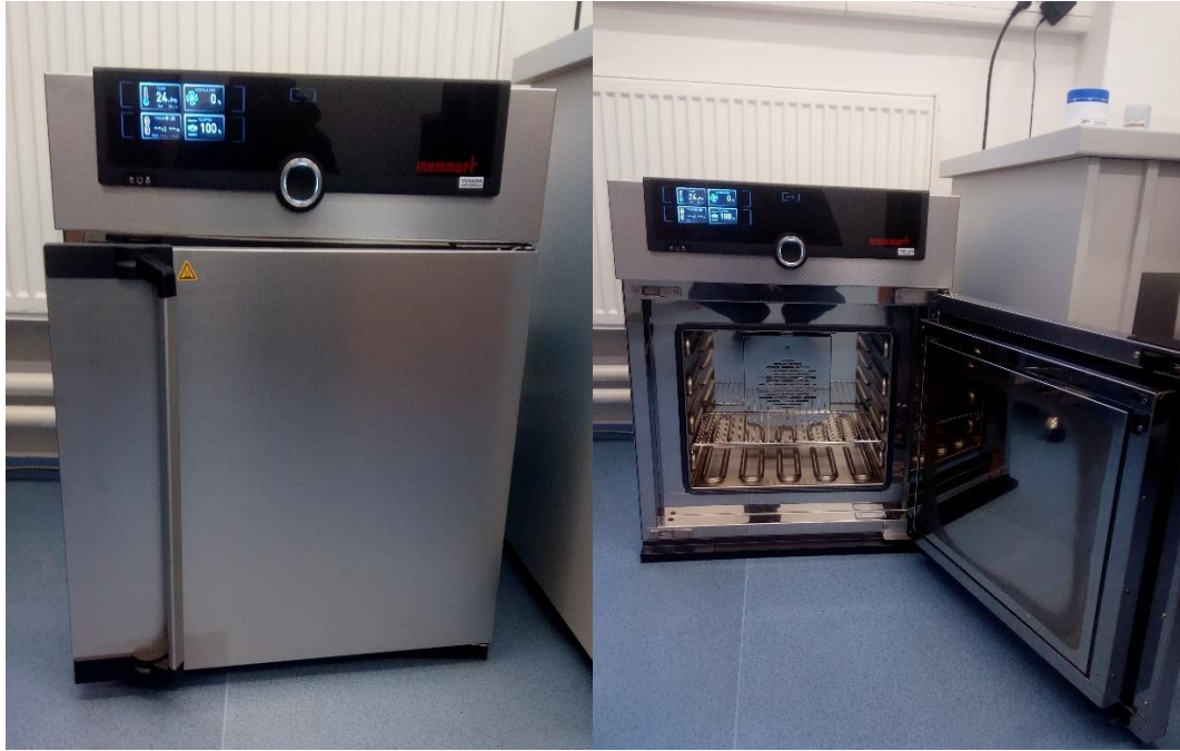
Figure 20. A caption of Laboratory Oven obtained during laboratory work at Faculty of Engineering, CULS
