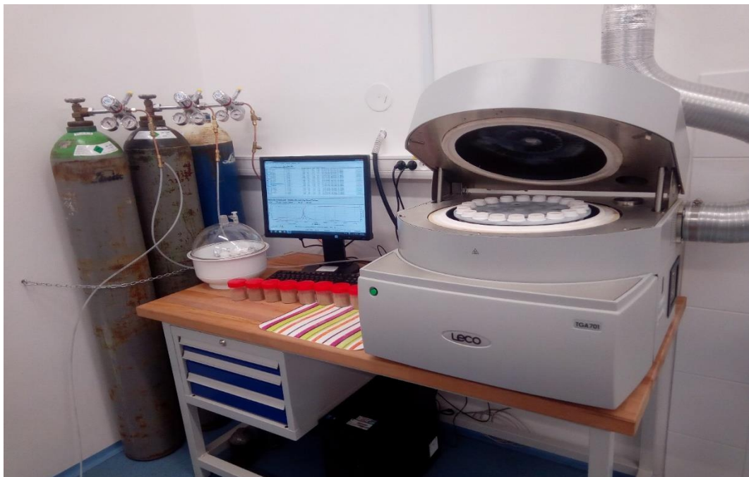
Figure 21. A caption of Thermogravimetric Analyzer (LECO TGA701) obtained during laboratory work at Faculty of Engineering, CULS
