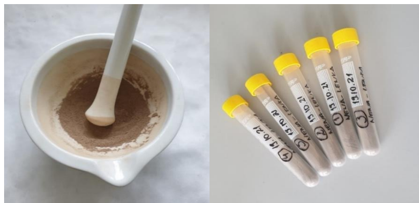
Fig. 22 Preparing soil for C/N analysis
