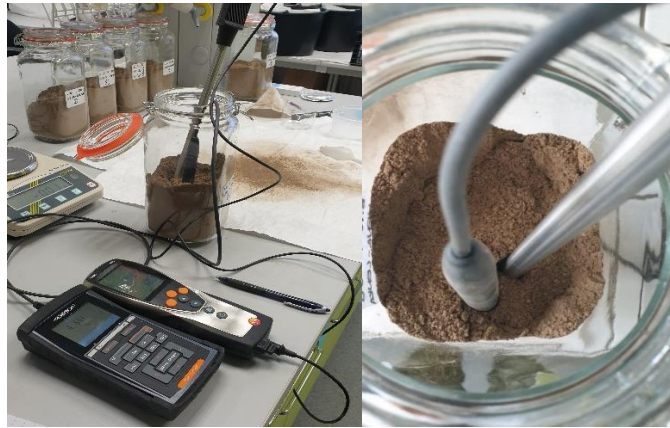
Fig. 21 pH and moisture measurements
