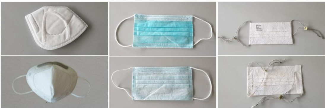
Fig. 14 Test material: a) respirator b) surgical face mask c) biodegradable face mask
