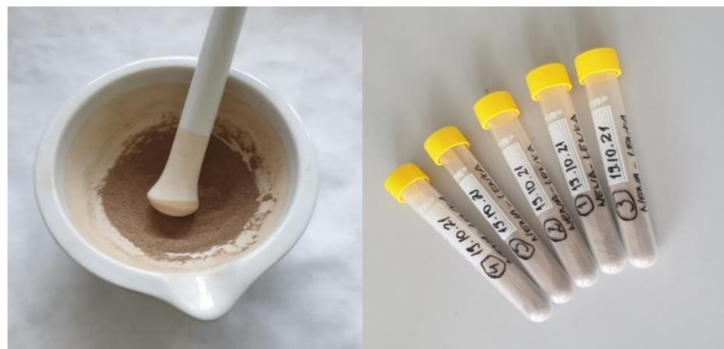
Fig. 22 Preparing soil for C/N analysis
