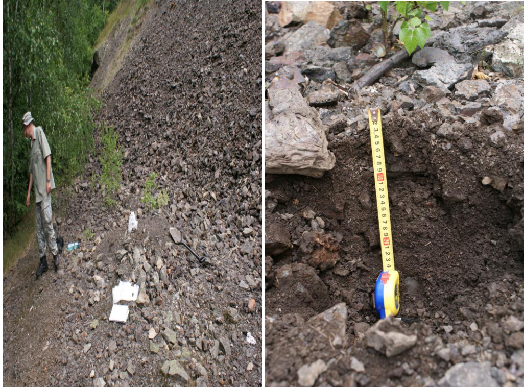
Figure D5 Area where loose slag was collected (left) and sample pit 3a (right)
