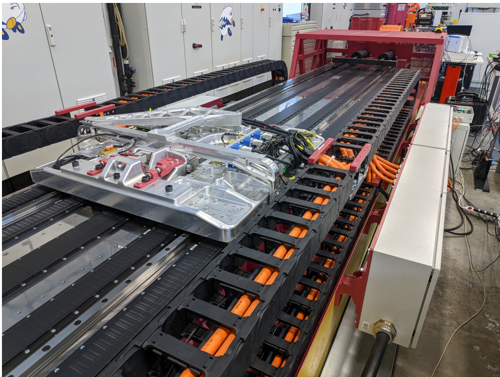
Fig. 7.10: Photo of used linear dynamometer.
