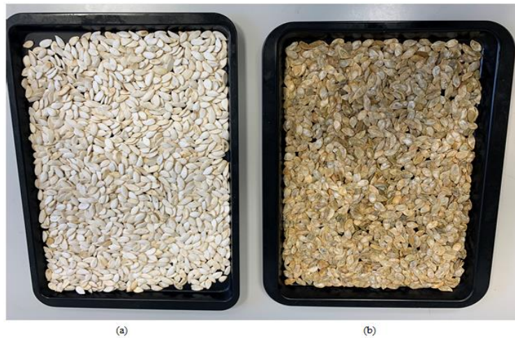
Figure 3. Pumpkin seeds before compression (a) and after compression process (b) for recovering the oil.
