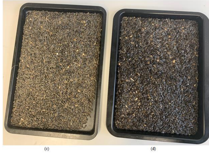
Figure 5. Sunflower seeds before compression (c) and after compression process (d) for recovering the oil.
