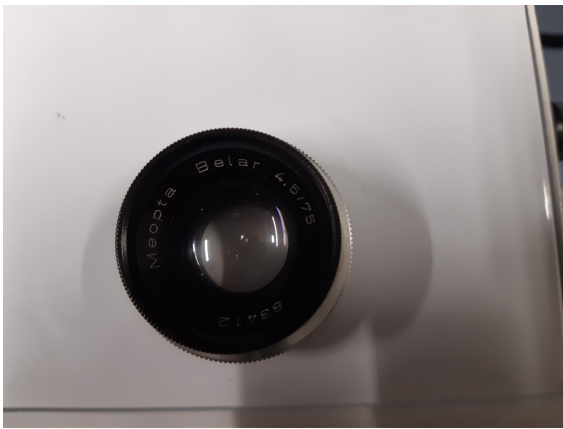
Figure 3.7: Microscope lens I used as an integrator.
