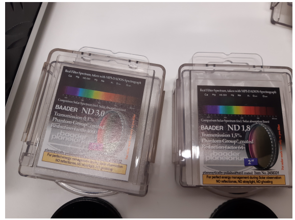
Figure 3.6: Gray filters used for attenuation of the beam for control over saturation.
