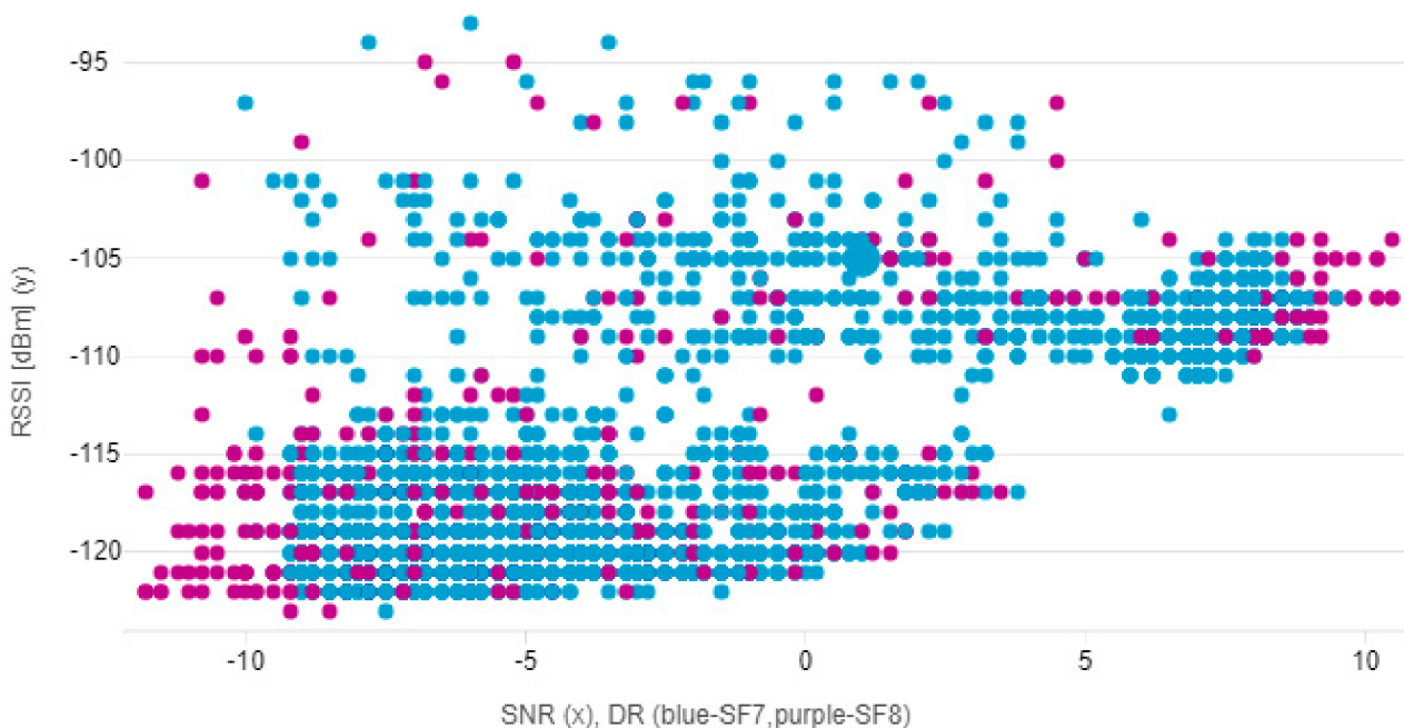
Figure 4. Scatter plot shows the relationship between signal strength and signal-to-noise ratio. The color resolution shows the currently selected spreading factor.
