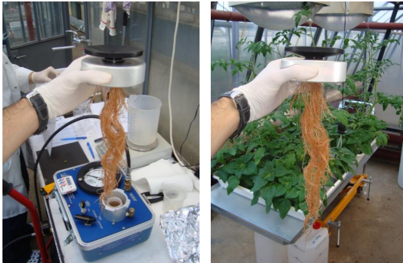
Image 4 L_o test using a Scholander chamber with each complete root system.
