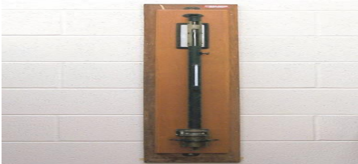
Figure 2 the mercury barometer (Robert, 2008)
