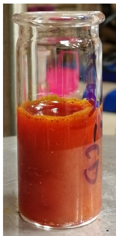
Figure 5.1: Photograph depicting the suspension of the \text{KAuBr}_4 complex with \alpha -CD.
