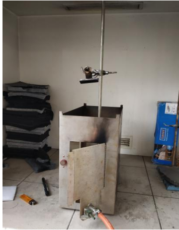
Figure 8. Flame test apparatus used for testing of flame behaviour.
