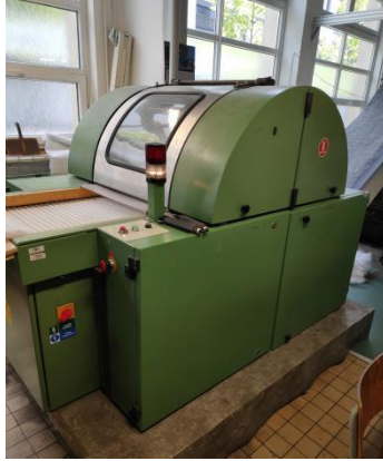
Figure 6. Carding machine used for manufacturing of nonwoven web.
