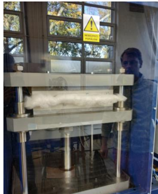
Figure 7. Hot press machine used for thermal bonding of the fibres.
