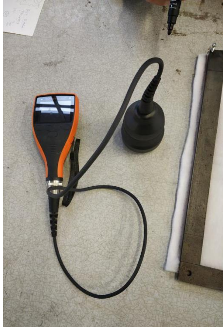
Figure 5. Thickness gauge used for measuring thickness of samples.
