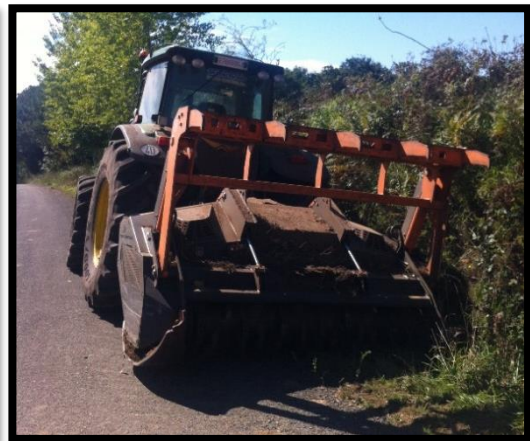
Photo 9. This is a bigger alternative of mulching machine for cleaning the higher shrub, stumps and also smaller trees with diameter of trunk until 25 cm approximately.
