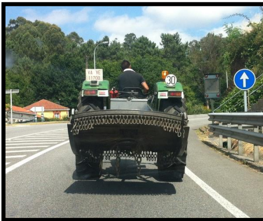
Photo 8. Photo of my colleague driving our small tractor with mulching machine behind. This equipment is enough for cleaning of small bush and grass.
