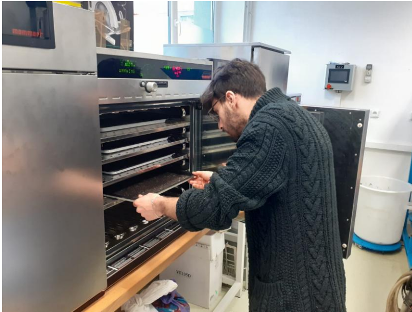
Figure 19. The student loading rapeseeds samples into the moisture conditioning equipment.
