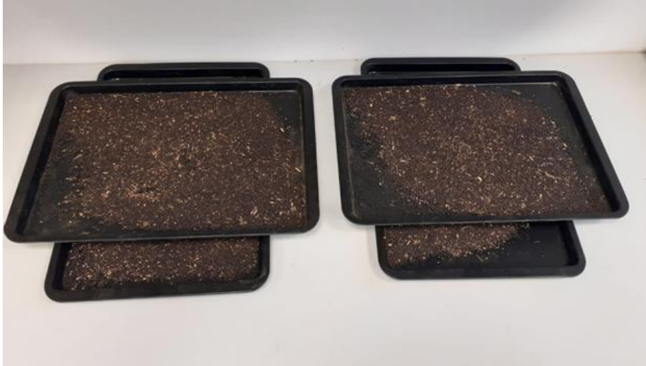
Figure 5. Rapeseeds sample prepared for moisture conditioning
