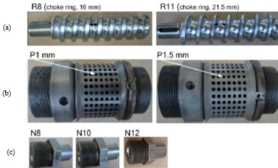
Figure 4. Independent variables of mechanical screw press Komet D85-1G. (a) Two different screws with choke worm shaft ring size 16 and 21.5 mm; (b) two different press cylinders with mesh size 1 and 1.5 mm and (c) three different nozzles with restriction size 8, 10 and 12 mm. Source: Karaj and Muller, 2011.
