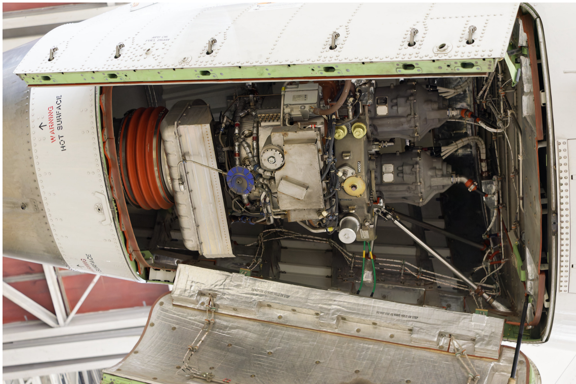
Obr. 1.4: Auxiliary Power Unit (APU) Boeingu 787 [10].
