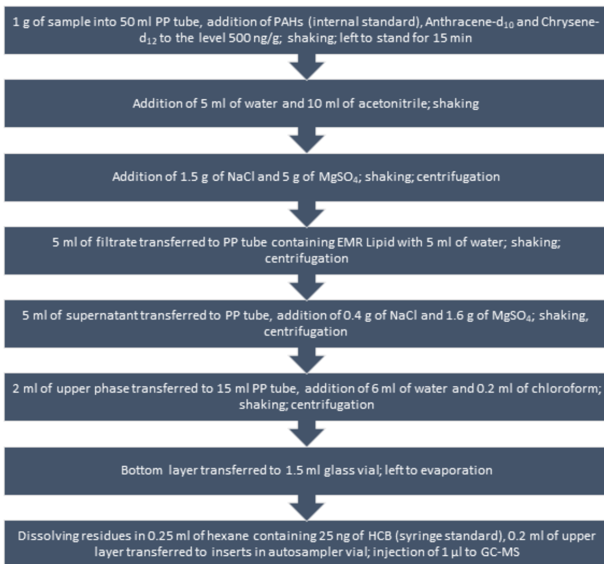
Figure 25 Schema of the sample preparation process; PP - polypropylene; centrifugation - 4 °C, 4.600 RPM, 15 min.
