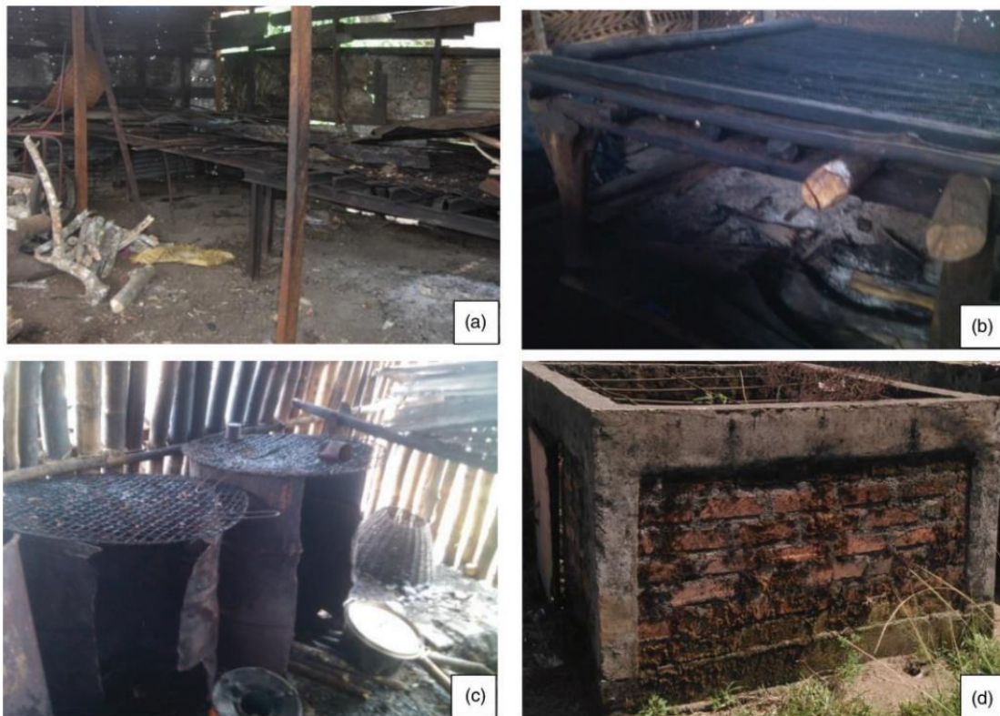
Figure 9 Oven types in study site. (a) Suspended iron banda. (b) Suspended wooden banda. (c) Circular oven. (d) Cinderblock oven (Dongmo Keumo Jiazet 2019)
