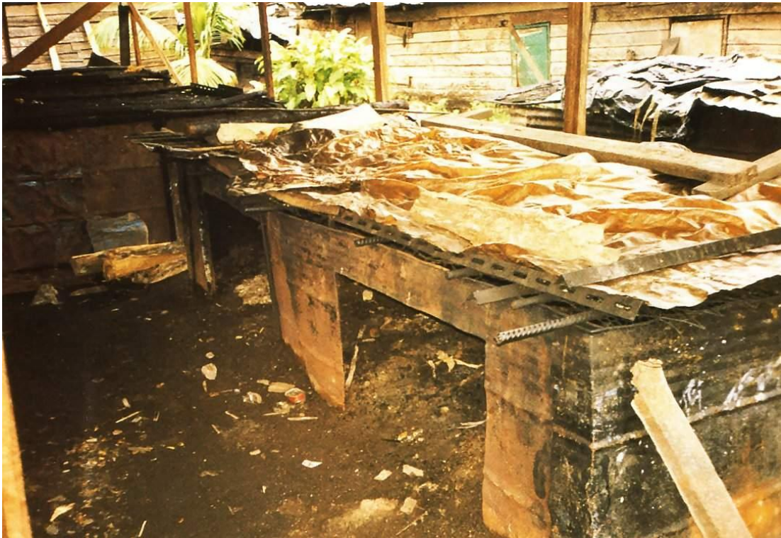
Figure 4 Closed banda kiln - Flattened barrel banda (FAO 1994)
