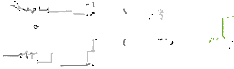
Fig. 5.4: Segmentation with an adaptive threshold - too distant objects. If no upper limitation for the adaptive threshold is specified, it becomes too permissive at large distances as depicted in the right side of the image. In such a situation, outliers may not be properly filtered out and cluster separation may fail as well.
