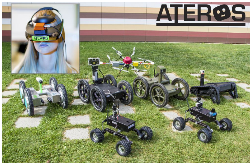
Fig. 4.5: ATEROS - the outdoor reconnaissance robots and an operator with a virtual reality head set.
