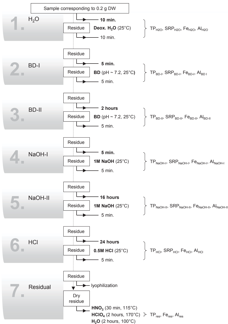
Figure 1. Sequential extraction scheme for determination of different forms of P, Fe and Al as modified from the original method by Psenner and Pucsko (1988).
