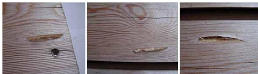
Fig. 10. The resin leak after 12 months of weathering at Siberian larch exposed to south side, construction type B.
