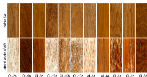
Figure 7. Visual changes of selected tested coating systems on oak wood. (OL-2a) the same degradation was observed using hydrophobic treatments b and c; (OL-9) positive effect of hydrophobic treatment (c) on color stability of AW samples; (OL-10) partly positive effect of hydrophobic topcoat application b and c; (AL-1) very similar degradation was observed using hydrophobic treatments b and c; (AL-4) positive effect of pigment content increasing durability of alkyd coating (in comparison with transparent (AL-1a)); (SL-1) positive effect of application of topcoat b; (SL-6b) positive effect of application of topcoat b.
