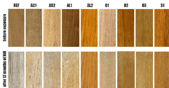
Figure 6. Visual evaluation of tested coatings before and after 12 months of NW exposure.
