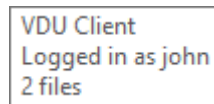
Figure 4.9: Example of a tray tip, shown above the icon when hovered, displaying the current state of the application.
