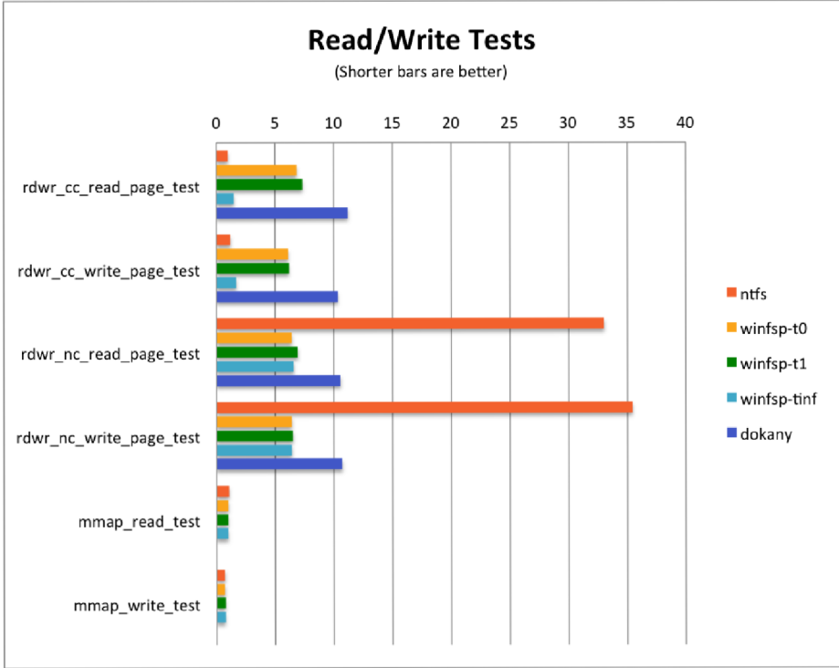
Figure 2.4: Performance comparison of read/write tests of WinFsp, Dokany and NTFS. Source:[48]
