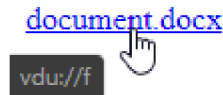
Figure 4.5: An example of a VDU URL protocol hyperlink, displayed on a website using an internet browser, which can be clicked to access a file with the token “f”
