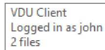
Figure 4.9: Example of a tray tip, shown above the icon when hovered, displaying the current state of the application.
