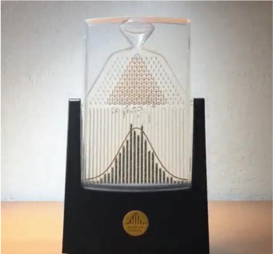
Picture 22. Example of a Galton board. The accumulated beads in the bins approximate the bell curve demonstrating the central limit theorem. [48]
