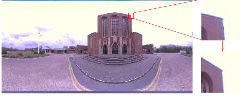
Figure 13: Correction of an extracted patch - From spherical latitude-longitude image (left) the corrected patch (right bottom) is computed using tangential projection.
