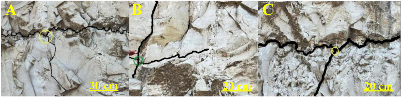
Figure 17 Stylolite Connectivity Stylolite connectivity analysis showing intersection angles and dimensions (A and C are Y types and B is a X type).
