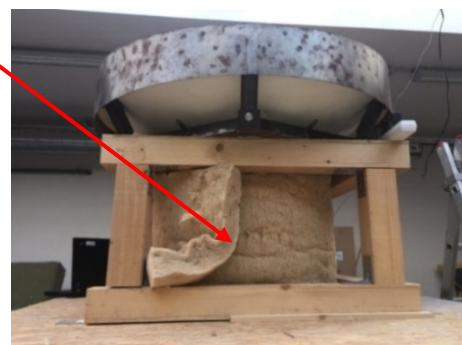
Fig. 3.26: Photograph of the light guide with additional thermal insulation (mineral wool)
