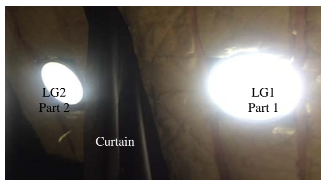
Fig. 3.32: Photograph of a view at LG1 and LG2 diffusers installed into the container's two identical parts, separated by black curtain
