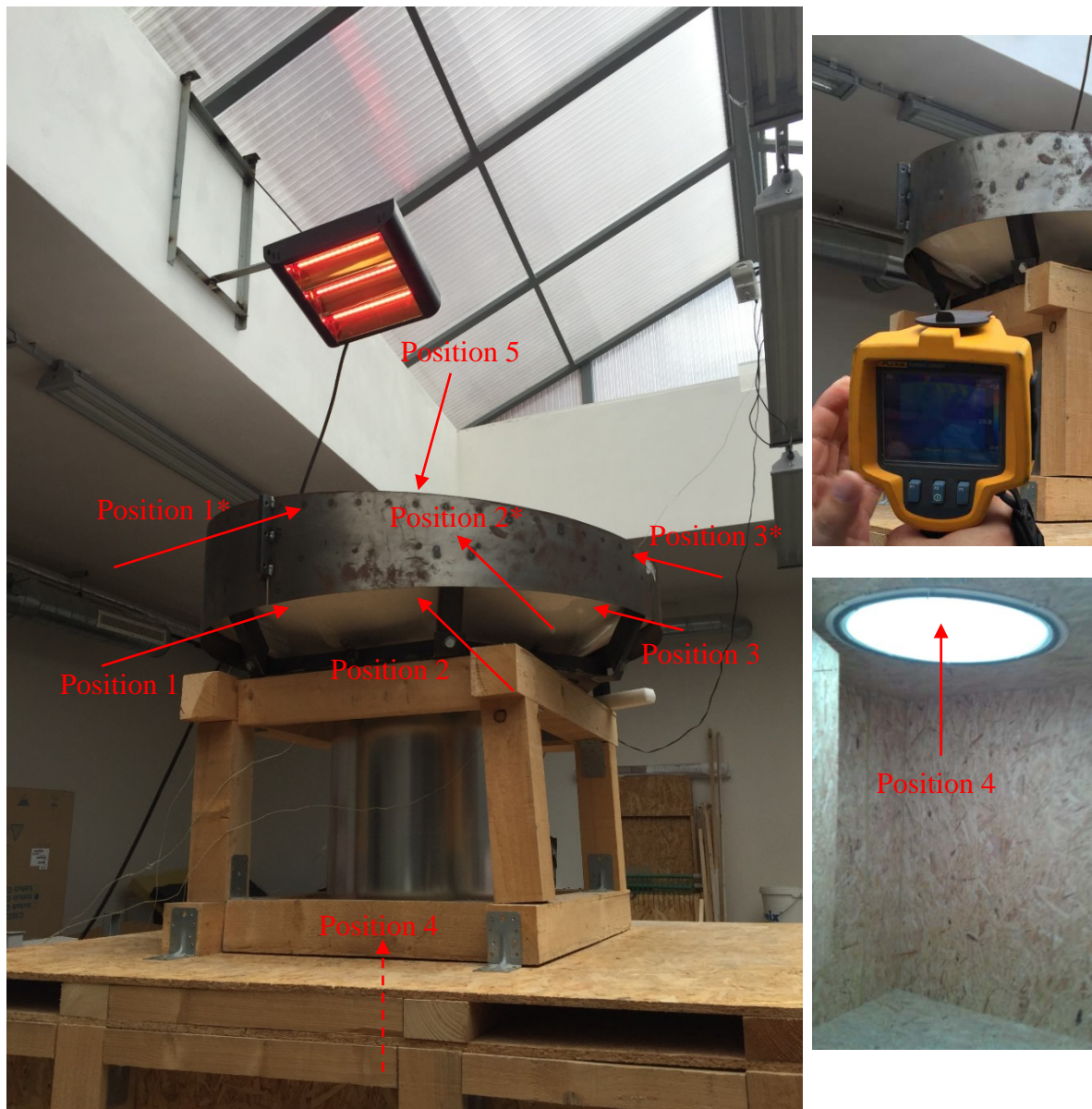
Fig. 3.24: Photograph of the light guide under the IR lamp radiation and view to the light guide diffuser (inside the chamber) (Positions 1, 2, 3 - directions of IR camera monitoring, position 4 – on the diffuser, position 5 - placement of IR lamp [40], positions 1*, 2*, 3* - on the metal rim of the light guide head).
