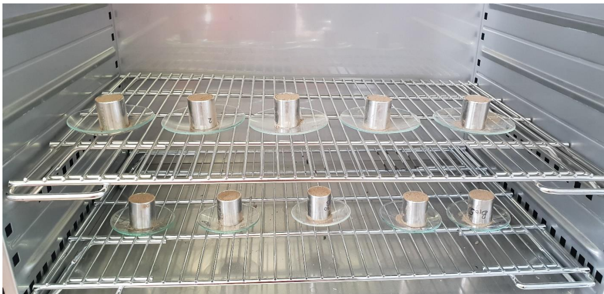
Appendix 15: Samples placed in oven at a temperature of 105°C for volumetric water content determination
