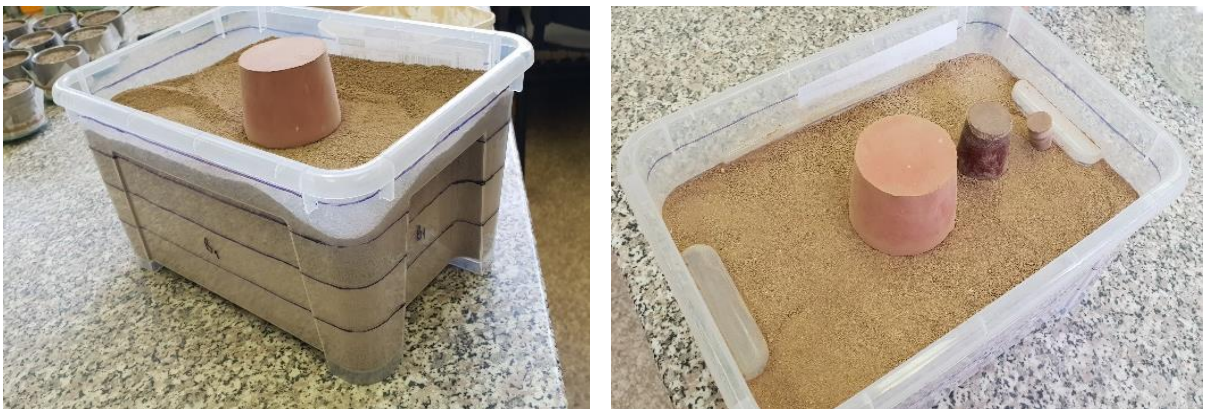
Figure 12: Calibration container with its layers and how the repacking was done in layers.
