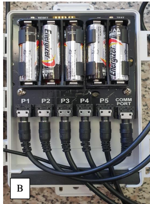
Appendix 7: (A) Exterior of EM50 Data Logger (B) Interior of EM50 Data Logger.
