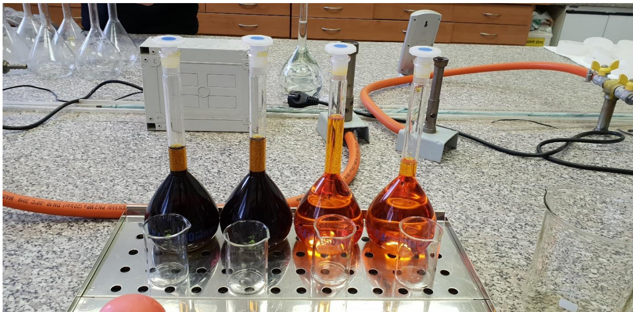
Appendix 5: Organic carbon content determination using a modified Walkley-Black method.
