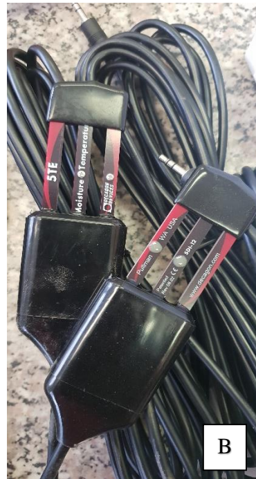
Appendix 9: (A) ECH 2 O EC-5 moisture sensor (B) 5TE moisture sensor.
