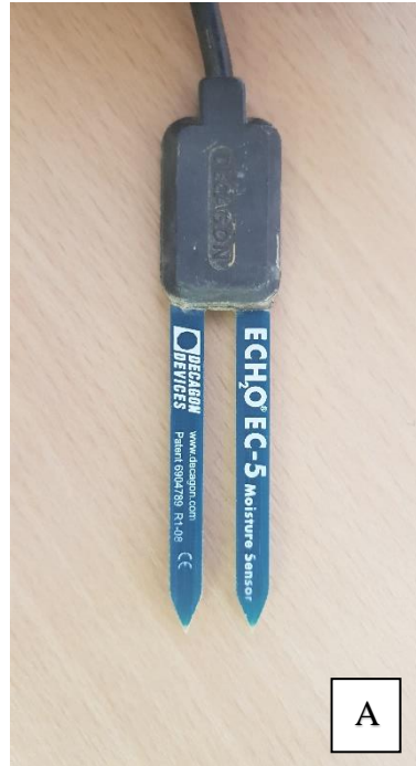
Appendix 9: (A) ECH 2 O EC-5 moisture sensor (B) 5TE moisture sensor.
