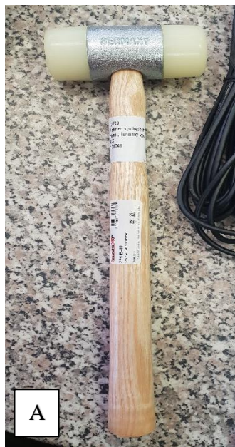
Appendix 10: (A) Hammer used for pushing the sampling rings into the soil sample (B) Sampling rings.
