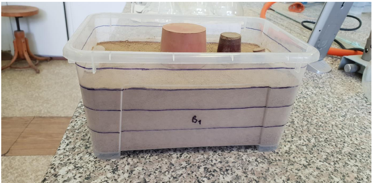
Appendix 12: Soil packed into the sampling bowl to the third level of desired bulk density.
