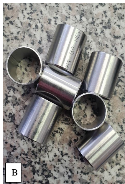
Appendix 10: (A) Hammer used for pushing the sampling rings into the soil sample (B) Sampling rings.
