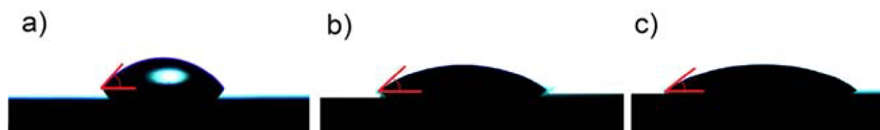
Fig. 46. Drop profiles PVA a), PVA/5%MFC b) and PVA/10%MFC c) on Bioglass ® substrates.
