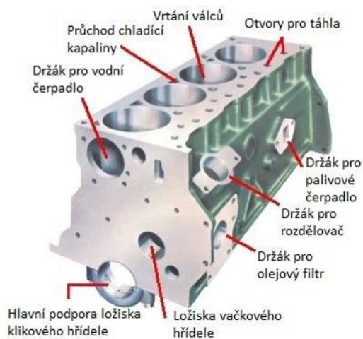
Obr. 10 Blok motoru, a) schéma bloku; b) Open-deck; c) Open-deck do tvaru V; d) Closed-deck
