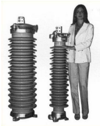
Fig. 3-1: Silicon Carbide Arrester on the left and MOV Arrester on the right, for 155 kV systems. 182 vs 91 kg. [2]
