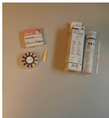
Figure 5: Equipment for urinalysis – Duotest ® pH-indicator papers and test strips for urinalysis DekaPhan ® Leuco (photo: author)
