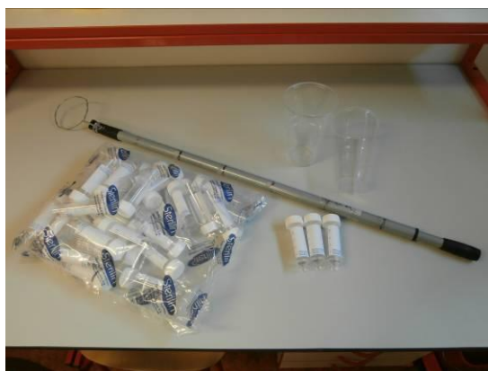
Figure 4: Equipment for collecting, transportation and storage of samples – a telescopic rod, plastic cups and containers (photo: author)
