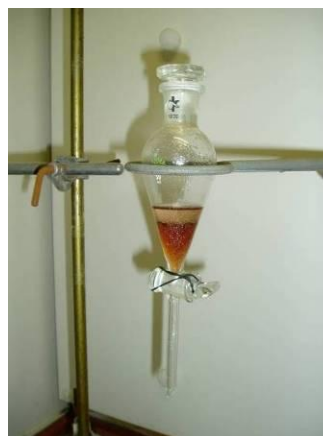
Separating of the toluene layer (photo: author)
