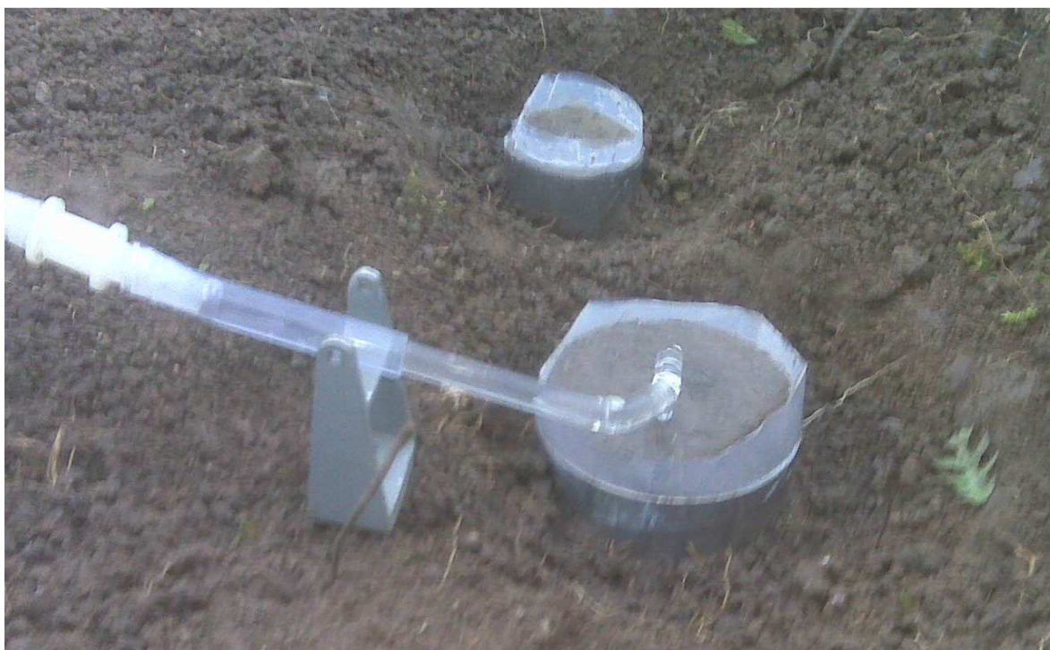
Figure 10. Constant water head maintained by plastic tape.
