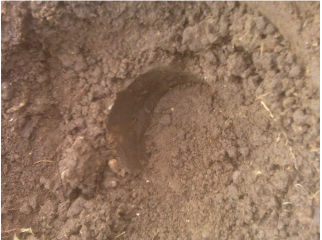
Appendix 6. No infiltration spot (small ring No. 005). There were not rock fragments. Thus it was a soil compaction factor.
