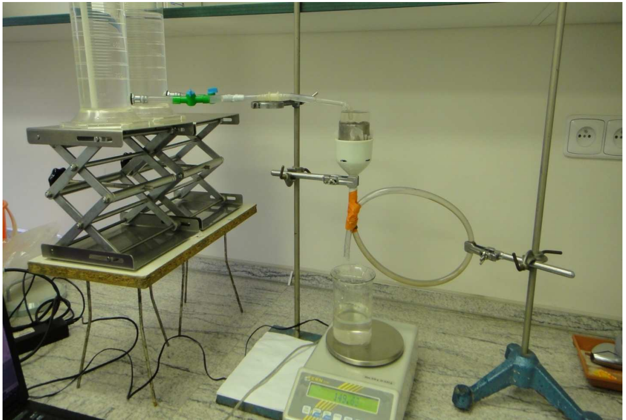
Appendix 2. Technical balance reading (connected to the Dasy Lab software)
