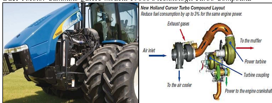
Obr. 4 Motor Cummins QSX15 modelu T9060 s technologií Turbo Compound
