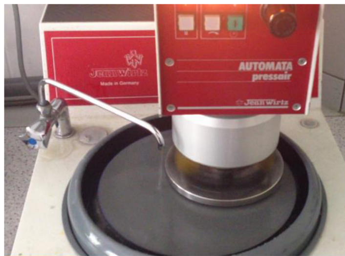
Fig. 3.22: The JeanWirtz TF250 in the process of polishing
