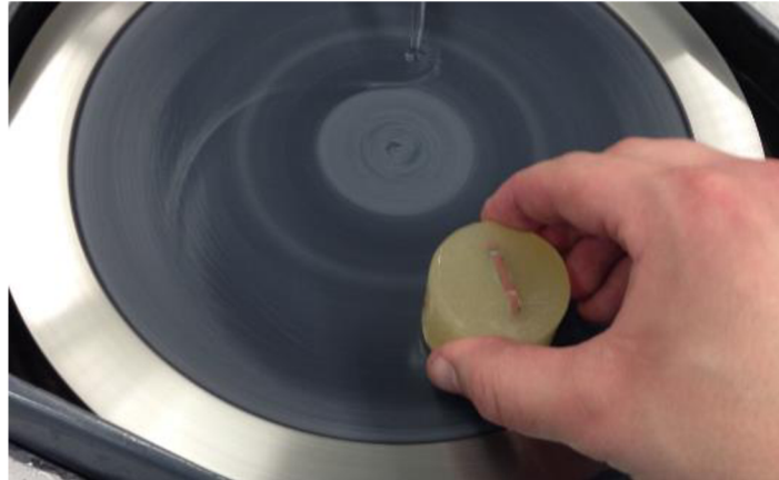
Fig. 3.19: Grinding the samples on rotary grinder
