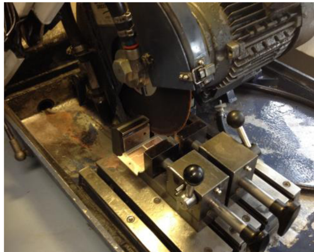
Fig. 3.21 : Metallurgical cutoff saw used for cutting the samples
