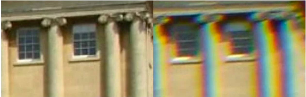
Figure 2.9: Example of lens distortion and chromatic aberration [23]
